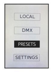
To store a group of settings, select the PRESETS menu option. Initially, the system presents 6 storage locations, labeled A-F. Turn the large knob to the desired storage location, push the large knob and the current settings for the fixture will be stored in that location. The unit automatically returns to LOCAL Mode.
