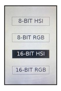
control values. If, for example the COURSE channel is set at value 165, the FINE channel adjusts between 165 and 166. Fortunately, most professional lighting consoles allow controls to be set up in 16-bit mode, so a single fader manages the two channels automatically. It is recommended that 16-bit mode only be used when the DMX controller supports 16-bit operation.
