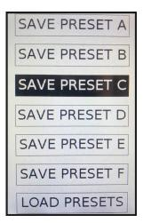
To recall a group of settings, scroll to the bottom of the SAVE PRESET list, and select LOAD PRESETS. The menu allows you to load any of the 6 stored presets by selecting it. Again, the unit automatically returns to LOCAL Mode.
